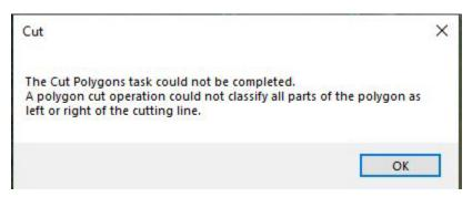
This error occurs because the polygon you are cutting out is not completely surrounded by edges of another selected polygon ("container polygon"). For example:
